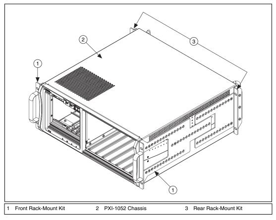
Figure A-3. PXI-1052 Rack Mount Kit Components
